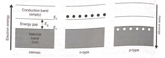
Fig. 3.3 Band diagram and electron-hole distribution in semiconductors
