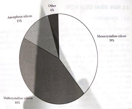
Fig. 3.1 Market share of the principal photovoltaic technologies (1998). 'Other' technologies include crystalline silicon cells for concentrator systems, cells based on ribbon silicon, cadmium telluride and silicon on low-cost substrates (Source: Paul Maycock, PV News)
